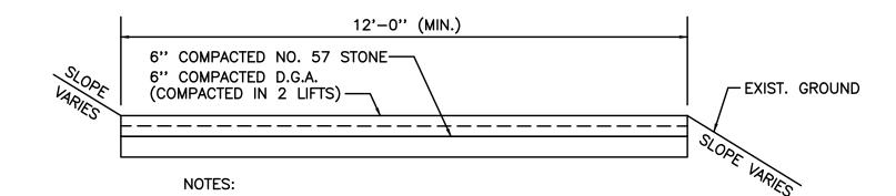
1. ACCESS ROAD TO BE SLOPED TO DRAIN.
